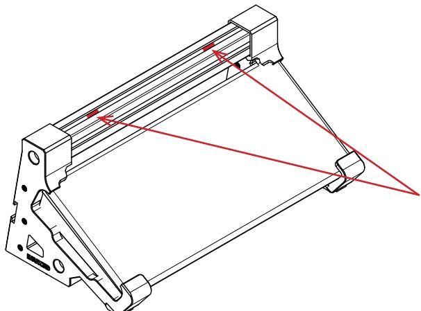
Position the Mini Stand as shown and note the 2x M4 slide in nuts you dropped in earlier
