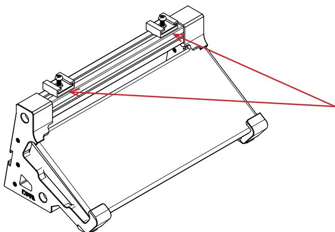
Place each cold shoe on top of the Mini Stand and **very loosely tighten** the 2x M4x8 bolts into the T-nuts
