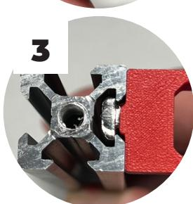
Attaching the cable managers requires the use of an M4x8mm bolt through the cable manager and into an M4 drop in nut.
