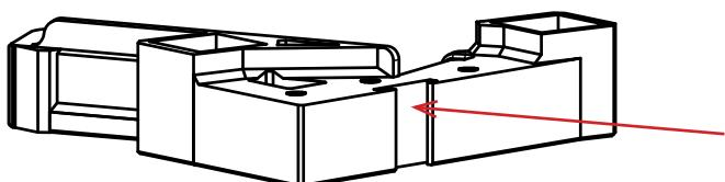
Begin by placing the left side of the Mini Stand smooth side down with the cold shoe facing you
